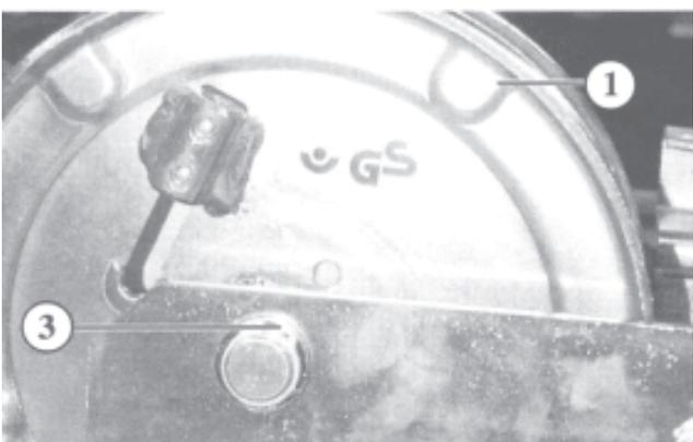
Fit the retaining ring (3) onto the drum axle
