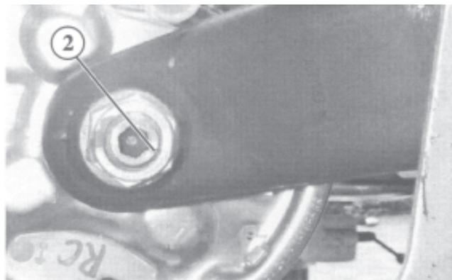
If corroded, clean up the threaded pin and end face
