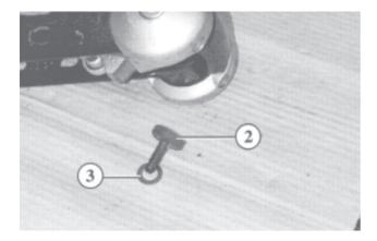
Press out the friction pads (2) inwards with a punch
