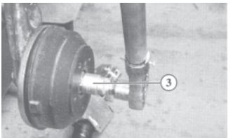
Tighten the new flange nut to a torque of 280 - 300 Nm (3)
