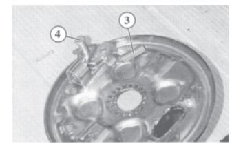
Hook a new tension spring (3) into the backplate by the square end of the spring Check that the automatic reverse lever moves freely
