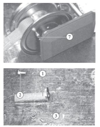
Insert and tighten the screw complete with washer (7) through the outside of the drum into the threaded hole in the anchor bar
