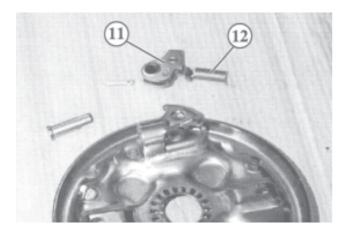
On the 1636 G wheel brake, the pivot bolt for the automatic reverse lever is riveted Drive the pivot bolt (10) inwards with a punch
