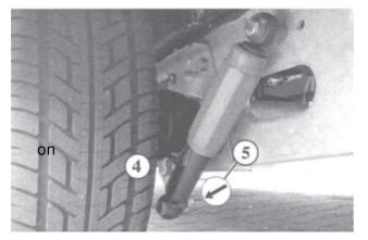
Fit the damper screw (4) on the correct side (shown here: inside fitting) of the damper mounting
