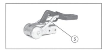
On the AKS 2000 with round side arms ([5], units built up to 1992), the AL-KO Safety cannot remain fitted for driving, as the stabilising handle cannot be operated fully ie the handle cannot be pushed fully down due to interference with the safety device..
