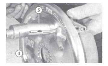
Push back the Bowden cable end bush (4) Lift off upper part (5) of the Bowden cable abutment
