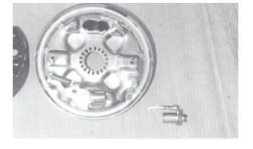
Grease the adjuster nuts and adjuster device Fit the adjuster device into the adjuster housing
