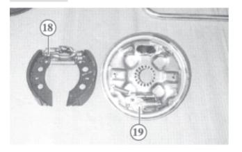
Ensure that the expander lever and automatic reverse lever are correctly positioned: the pivoting point of the expander lever (18) must be fitted on the same side as the pivot bolt of the automatic reverse lever (19)
