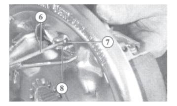
Push the Bowden cable (6) into the backplate so that the nipple (7) can be released from the attachment eye (8) Pull out the Bowden cable
