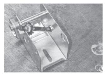
Press the bearing bush (5) outwards and remove
