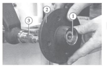
Insert the greased taper roller bearing (1) and DIN washer into the wheel hub (2).
