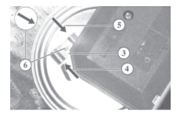
Pass (4) the cable end out of the opening and under the retaining plate (3) Bring the cable end back to the other side of the retaining plate (5) so that a semicircular loop is formed Tighten the screw (6)
