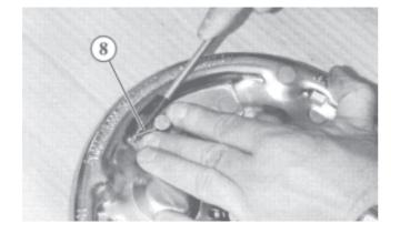
Insert and bend over the split pin (8) securing the pivot bolt
