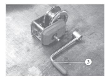
Loosen and take off the crank handle (3) by turning to the left several times
