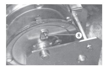
Tighten the self-locking nut (8) on the outside of the drum
