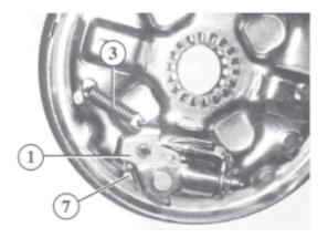
The automatic reverse lever (1) must be against the stop of the adjuster housing (7)
