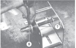
Fit the crank mounting (7) onto the drive shaft Drive a new pin (8) into the drive shaft
