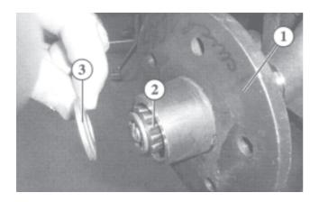
Pull off the wheel hub together with the taper roller bearing (2) inside it, and also the DIN washer (3) Pull out the taper roller bearing and clean
