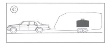
The correct condition is to load the trailer centrally as far as possible, making full use of the permissible drawbar load (figure C).
