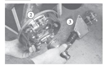
Unscrew the nut or socket head screw
