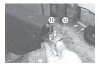
• Loosen and unscrew the nuts of the screws (11)
