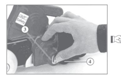
Press in the lock barrel (3) until it engages Dust is excluded by the cover (4) which swivels over the lock barrel. Close the stabilising lever
