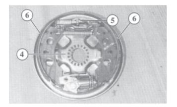
The backplate (4) is rigidly fitted or welded to the swinging arm and does not rotate. When the brake is applied via the Bowden cables, the expander (5) presses the brake shoes (6) against the brake drum. The vehicle is braked.
