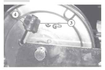
Pass the cable end out of the opening and through the sleeve (3) Tighten the screws (4) on the outside of the sleeve
