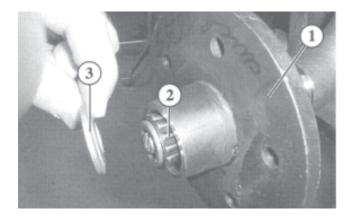
Pull off the wheel hub together with the taper roller bearing (2) inside it, and also the DIN washer (3) Pull out the taper roller bearing and clean
