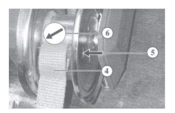
Pass (5) the anchor bar from the outside of the drum through the strap loop (4) Engage the anchor bar on the opposite side (6)
