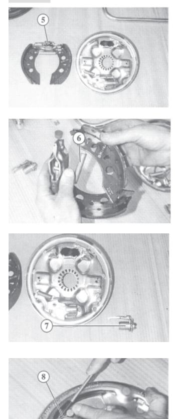
Take off the brake shoes with expander lever and return spring (5)
