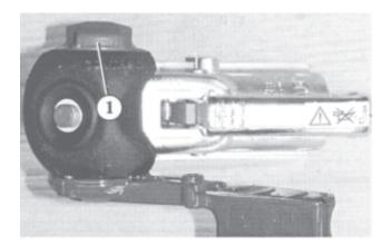
The marking "zu" [closed] (1) must be visible on the AKS 2000/2500/2700.
