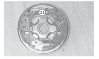
Pass the brake shoe steady spring clips through the openings (21) in the brake shoes
