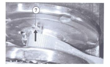
From the inside of the drum, insert the carriage bolt (7) into the square opening in the anchor bar
