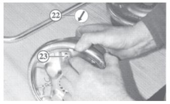
To secure, press the brake shoe steady spring (22) towards the backplate Push in a new cover plate (23) (the plate may be omitted in the compact axle service)
