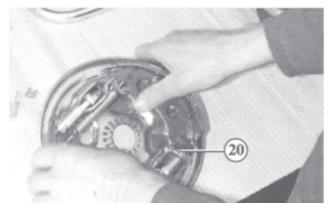
Place the assembly of brake shoes, expander and tension spring onto the backplate.
