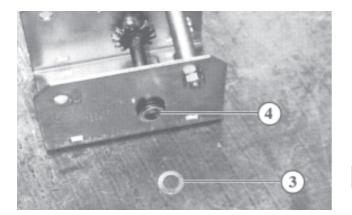
Remove the retaining ring (3) from the drive shaft
